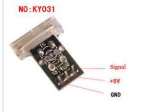
Knock sensor module and a digital interface, built-in LED build a simple circuit to produce percussion flasher. Interface comes with digital LED, will knock sensor connected digital 3 interface, when percussion sensor senses measure to percussive signals, LED flashing light.
