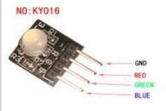
This is a through the hole three-color LED module that can make any color we want by combing different intensities of Red, Blue and Green.
