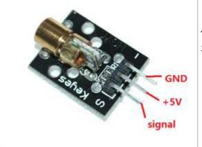
This is a laser emitter diode. The working voltage is 5V, with a wavelength of 650nm.
