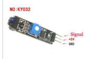
Obstacle avoidance sensor module KY-032 for Arduino: With 4 pins, use an infrared beam to detect proximity of obstacles. The potentiometers can be used to adjust sensitivity. Pin 1 is Ground, pin 2 is 5V power, pin 3 is digital output (on/off depending on the beam), 4 is enabling.
