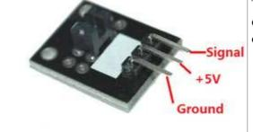
This is a light block sensor module, where there is an object in the middle of the U shape. The sensor will output a high level signal.
