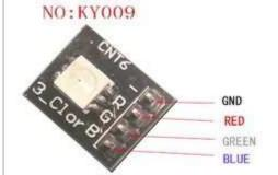
This is a surface mount three-color LED module that can make any color we want by combing different intensities of Red, Blue and Green.
