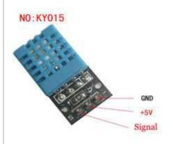
This DHT11 Temperature and Humidity Sensor features a calibrated digital signal output with the temperature and humidity sensor complex, ensureing the high reliability and excellent long-term stability. A high-performance 8-bit microcontroller is connected. This sensor includes a resistive element and a sense of wet NTC temperature measuring devices. It has excellent quality, fast response, anti-interference ability and high cost performance advantages.
