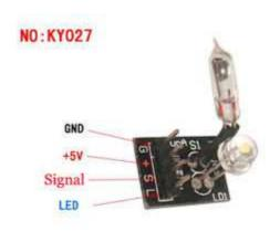
This module has two parts - an LED and a mercury tilt switch. Pins are 1 G (ground), 2 + (5V power), 3 S signal and 4 L (LED.) If you wired up 1 & 2 to power, pin 3 (signal) will alternate between 5V (HIGH) and 0V (LOW) as you tilt the module. If you connect a current limiting resistor to L2, you can use it as a blinking LED.
