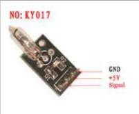
A tilt switch that can turn on and off depending on the tilt position. The switch is mercury.
